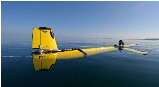
A data-gathering glider used by EPA scientists on underwater missions that can last up to 100 days.
